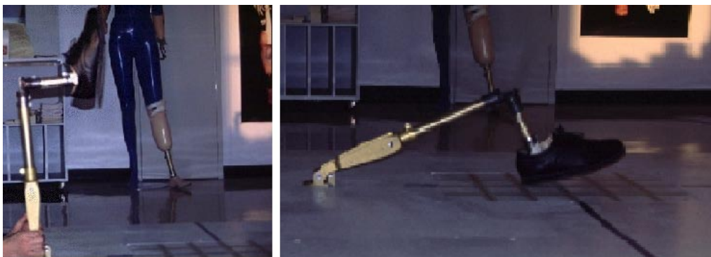
Picture 1: Impact testing apparatus with the e-shoe in starting (left) and final (right) position
