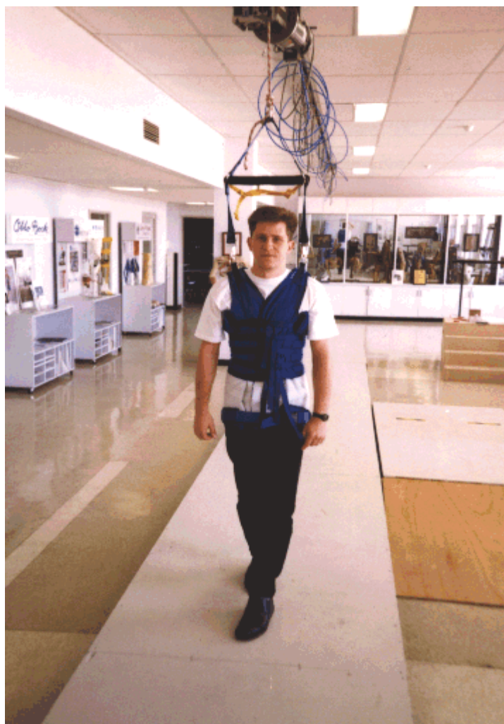
Figure 36. Overhead harness system and walkway
