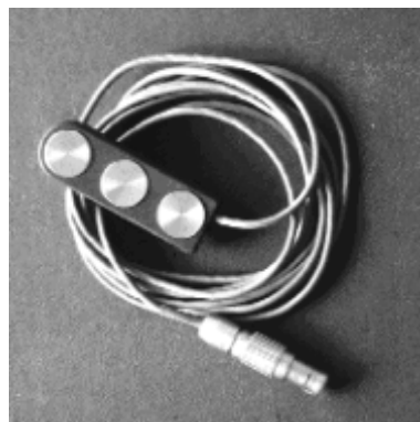
Figure 4.1. Surface electrode used to measure EMG activity.
