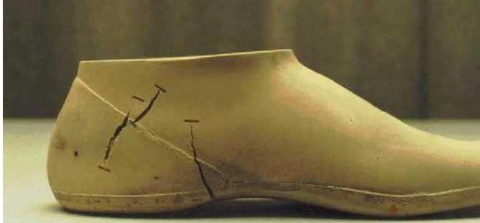
Figure 4.3. Kingsley SACH - 20,000 cycles. (Note deep cracks medially)
