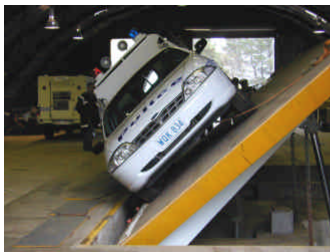
Figure 3 View showing vehicle undergoing Tilt table test at Monegeetta
