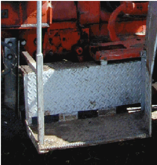
Figure 1. Positioning of steps with respect to driver platform and mudguard width (safe tractor access platform evaluation, Victoria, 2001–2002).
