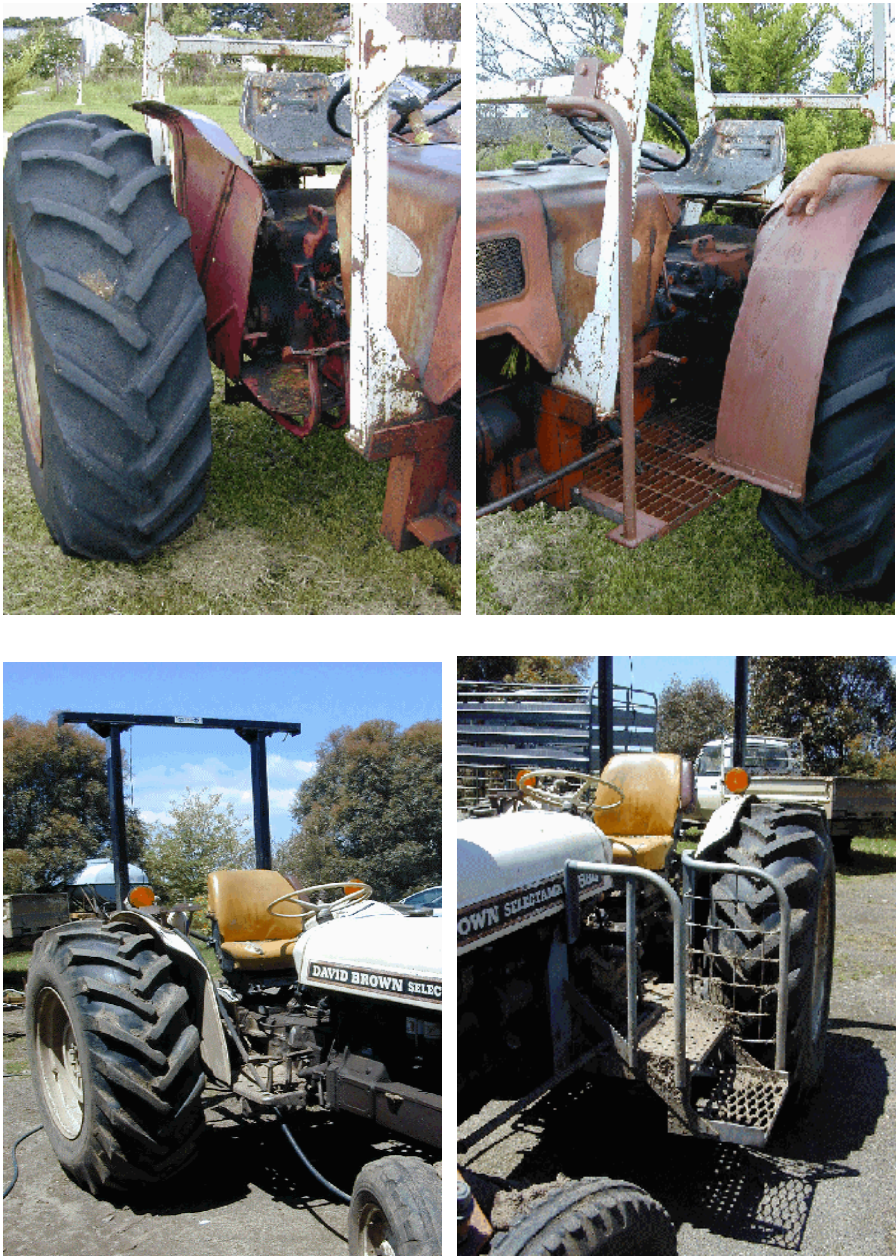
Figure 3. Examples of (left, top and bottom) pre-retrofit and (right, top and bottom) post-retrofit tractors (safe tractor access platform evaluation, Victoria, 2001–2002).
