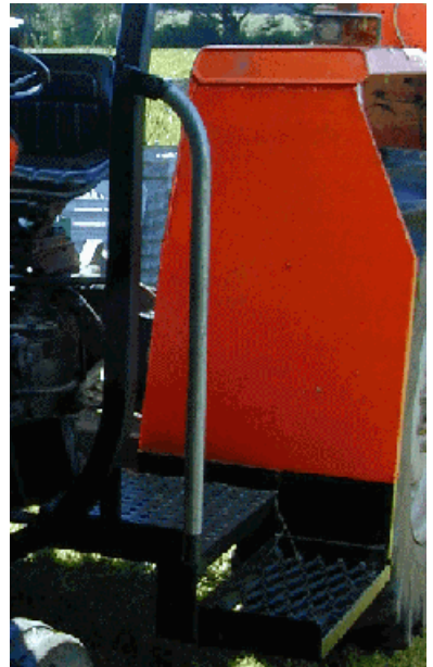
Figure 1. Positioning of steps with respect to driver platform and mudguard width (safe tractor access platform evaluation, Victoria, 2001–2002).
