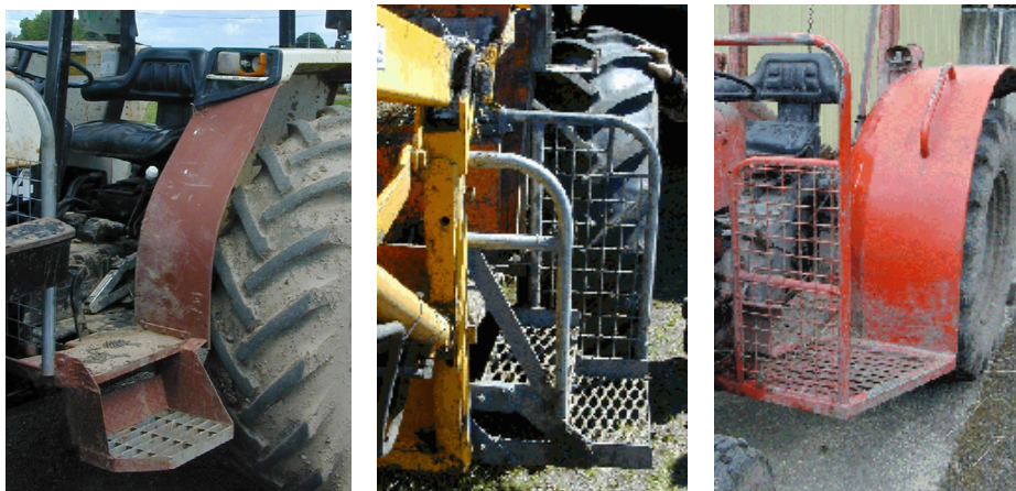
Figure 2. Examples of guarding of rear wheel: (left) incomplete guarding of rear wheel, (middle) complete guarding of rear wheel by rear handrail and wire mesh, and (right) complete guarding with mudguard (safe tractor access platform evaluation, Victoria, 2001–2002).
