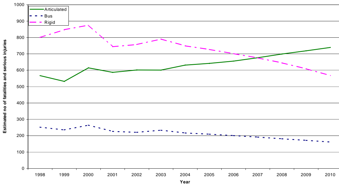
Figure iv. Estimated number of fatalities and serious injuries resulting from collisions between heavy vehicles and light passenger vehicles where articulated truck travel is restricted to non-metropolitan areas; Linear forecast of crash rates.
